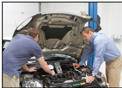
Bentley technical editors testing fuel pump on the Cooper S engine.
