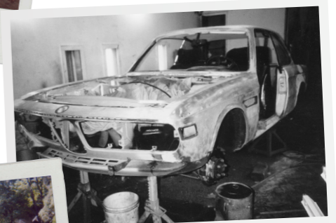
Rob's 1973 BMW 3.0CSi stripped to bare metal during its outer body restoration. (Photo by Rob Siegel)
