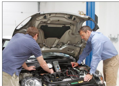
Bentley technical editors testing fuel pump on the Cooper S engine.
