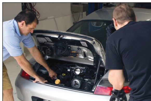
Bentley technical editors removing drive belt prior to servicing a 3.6 liter Carrera coupe.
