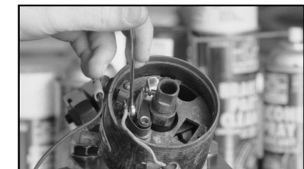
On the bench, the condenser and points come out easily. Old Autolite point sets have one hold-down screw. The breaker arm pivot slides over a support pin on the breaker plate.
