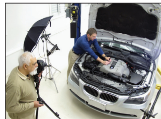
Bentley technical editors removing motor cover on V8 (N62) engine.
