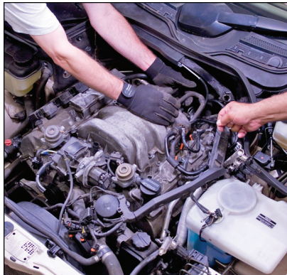
Bentley technical editors removing intake manifold on V6 (M 112) engine.
