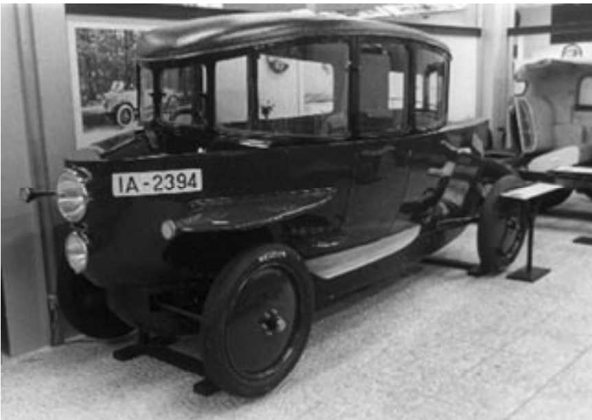
In 1921 the Austrian engineer Edmund Rumpler, working in Germany, introduced the world's first aerodynamic rear-engine production car. The Rumpler Tropfen-Auto inspired rear-engine production cars at Benz and later Mercedes-Benz.
