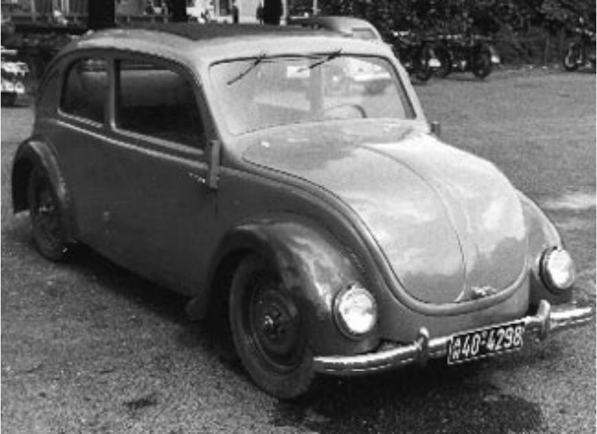
Porsche's small-car prototype for NSU, the Type 32 designed in 1933 foreshadowed the main features of the Volkswagen with its torsion-bar springs and air-cooled flat-four engine. Its body shape would become familiar as well.
