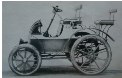
Chapter 1: Porsche's system of electric motors integral with the driving wheels required those wheels to be relatively small to achieve a high enough rate of motor revolutions in relation to vehicle speed.
