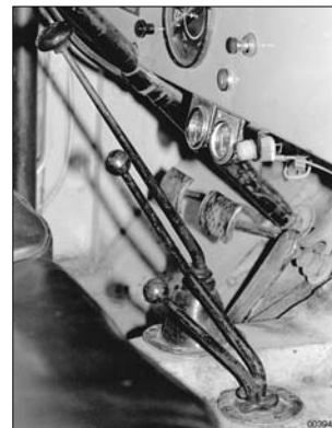
Fig. 10-24. Mechanical clutch linkage requires regular inspection for wear and excessive play. Models with through-the-floor pedals have the advantage of chassis mounted linkage. This reduces the tendency to flex, distort and bind. From Chapter 10 - Clutch and Transmission Service
