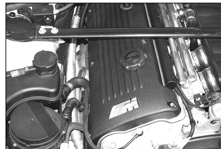
Maintenance and service, including checking and adjusting valve clearance on the S54 M3 engine 130 Fuel Injection
