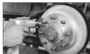
Non-directional finish of rotors assures semi-metallic lining break-in. Some manufacturers recommend a brake lathe grinder for this task, while others find a hand held drill motor and disc sander acceptable. Use a particle mask and safety goggles.
