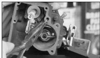
Check balls, needles and other sensitive parts need careful handling. Note that pliers grip the needle away from the tapered tip.
