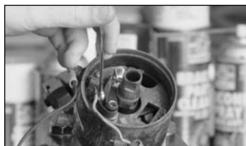
On the bench, the condenser and points come out easily. Old Autolite point sets have one hold-down screw. The breaker arm pivot slides over a support pin on the breaker plate.
