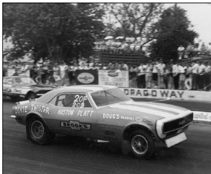
Chevrolet drag racers loved the Camaro for its big engines and light weight. This Camaro "funny car," the Dixie Twister, was actually a fiberglass body on a welded tubular frame. Here driver Huston Platt sticks it to Tasca Ford's Single Overhead Camshaft 427. courtesy Gold Dust Classics
