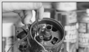
On the bench, the condenser and points come out easily. Old Autolite point sets have one hold-down screw. The breaker arm pivot slides over a support pin on the breaker plate.
