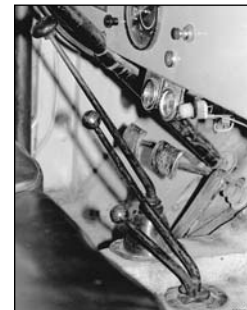
Mechanical clutch linkage requires regular inspection for wear and excessive play. Models with through-the-floor pedals have the advantage of chassis mounted linkage. This reduces the tendency to flex, distort and bind.
