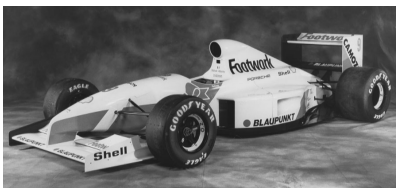
Chapter 53: The Arrows FA12 weighed in at the class minimum weight of 500kg despite an overweight and underpowered engine.
