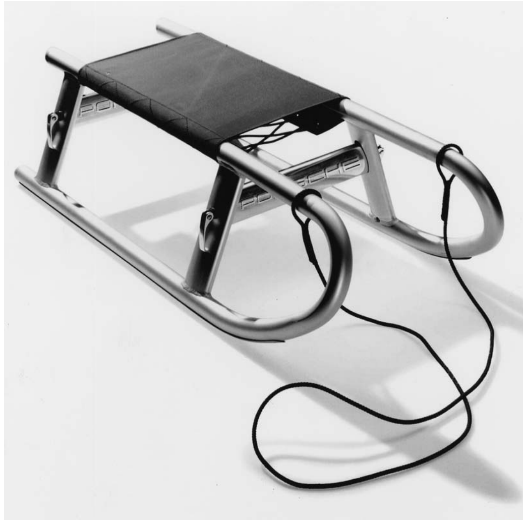
Constructed of tubular aluminum with steel runner surfaces and a stretched and laced nylon top, the Porsche sled could be folded and carried in a convenient nylon case.
