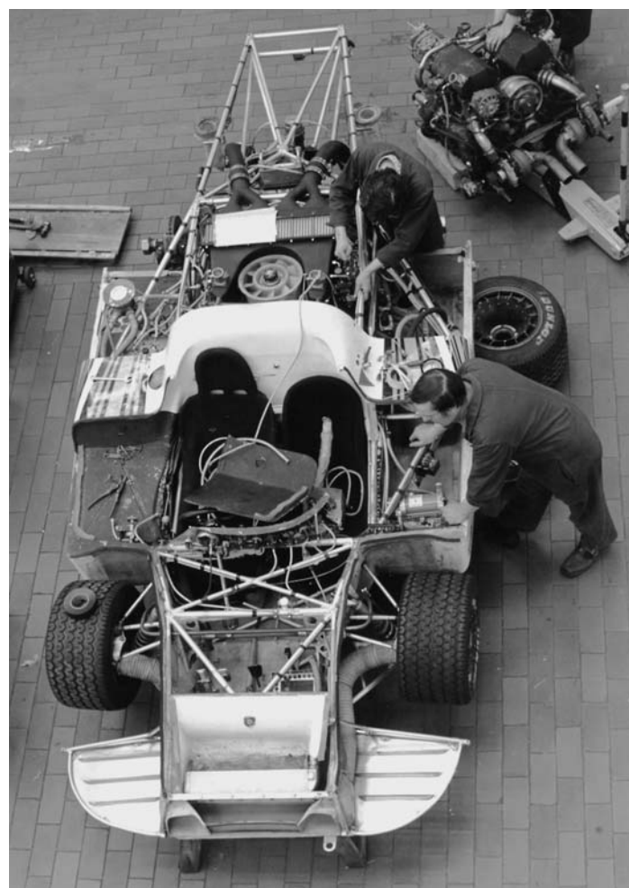
Top: Porsche optimized its 936 for the 1977 running of Le Mans with reduced frontal area, a lower drag factor and twin turbos instead of the single unit used in 1976.
