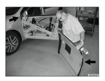
Outer door panels are removable for servicing components inside door cavity
