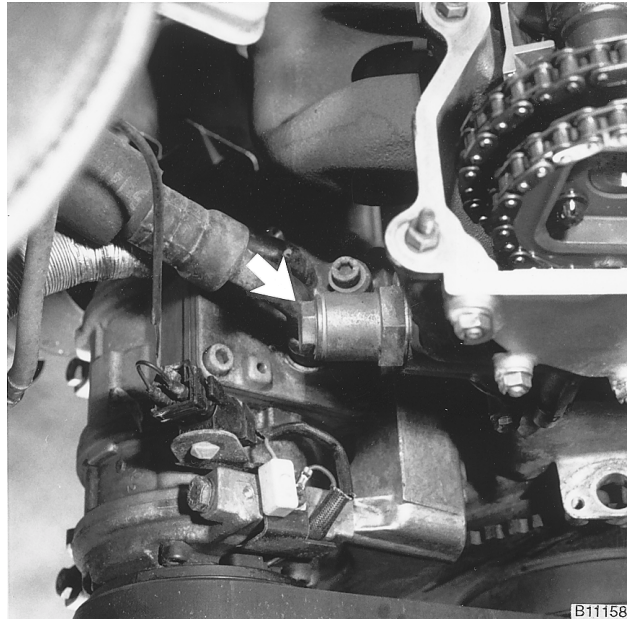
Fig. 40. Primary timing chain tensioner (arrow). Remove tensioner slowly to relieve spring tension beneath end plug.
