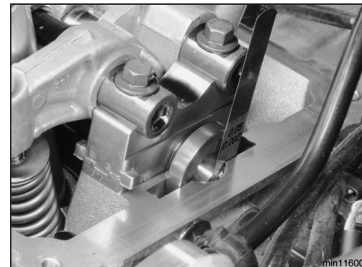
Measuring camshaft axial play. 116 Cylinder Head and Valvetrain
