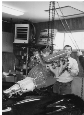
Lowering the engine with the transmission installed necessitates standing the assembly on end, but it can be done. Secure lifting equipment, patience, and steady hands are essential.
