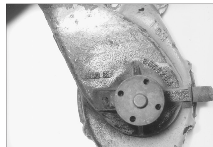
(1) Overall view of #3703524. (2) This photo shows the casting number H 18 5 (Aug. 18, 1965). Most Corvette water pumps use these types of casting dates.
