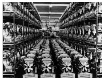
Stocks of the all-alloy, twin-cam engines await installation in new Alfa Romeo Giulias.
