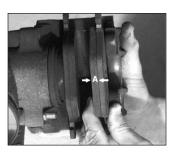
See how to perform routine maintenance procedures, such as checking brake pad thickness. 020 Maintenance
