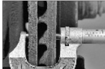
Measuring brake rotor wear. 00.04 Maintenance
