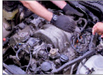
Bentley technical editors removing intake manifold on V6 (M 112) engine.
